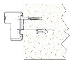
12. Unscrew and remove the cap head screw, leaving the frame fixing in the wall. Working through the frame access hole, move the sliding washer plate across, so that its 10.5mm hole is concentric with the 16mm frame tray hole.
