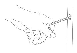
3. Tighten the frame adjusters clockwise, with a 5mm ball-ended Allen key, until the ends of the spreader plates are flat against the wall.
