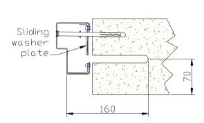
10. Ensuring that the sliding washer plate is away from, and not covering the 16mm frame tray holes, drill through the access holes in face 2 with a 15mm masonry bit to a depth of 160mm.
