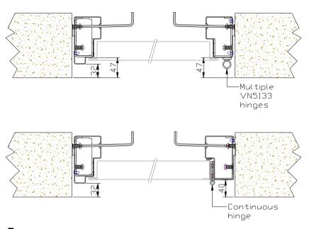
**5.** Set the lock jamb back into the wall a minimum of 32mm, to avoid the fixings breaking out of the wall later.
